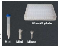
Fig. 1: Available formats of S-Traps™. Micros handle < 100 µg, minis and the 96-well plate 100 – 300 µg and midis > 300 µg.
